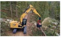
faster. High Wide undercarriage provides 15% greater ground clearance to help the machine pass over stumps and other obstructions with ease.
