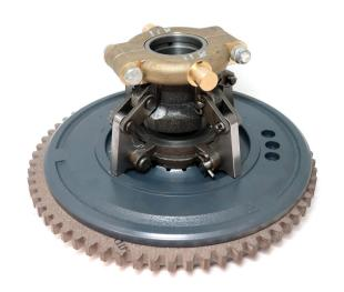
Foley Engines now offers both new and factoryremanufactured power take-off (PTO) clutches with upgraded severe-duty components, including 100% Kevlar composite discs. These proprietary Kevlar composite linings are designed to have as much as a 300% longer service life, compared to the molded-fiber friction discs commonly used, and to avoid failures caused by broken teeth. The firm specializes in Twin Disc/Rockford and WPT Power clutches.
