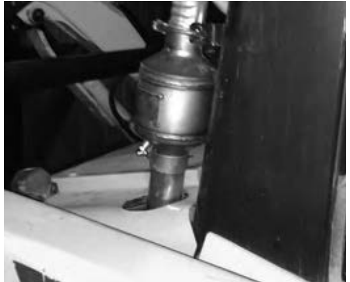
A custom scrubber made at Foley's Worcester, Massachusetts, plant.
