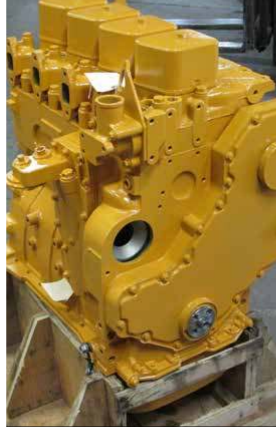
Cummins 4B engine for use in an irrigation pump.
