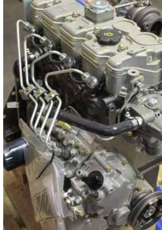
New Perkins replacement engine for CAT 277 Skid Steer.
